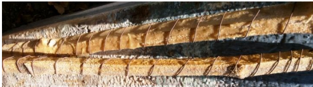
Figure 2. Treated Bamboo Specimens with Winding.
